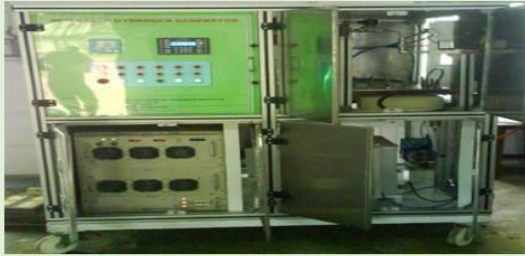
PEM Water Electrolyser Unit (1 Nm 3 /h)
